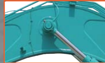
Reinforced boom center boss
